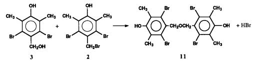
In electronic encapsulation and laminate applications, the *m*-bromobisphenols synthesized above have exhibited superior hydrolytic and thermal stability as compared with the conventional *o*brominated bisphenols. These properties have resulted in an extended device life for semiconductors and the printed circuit board, while meeting flame retardancy requirements as well.<sup>5</sup>
